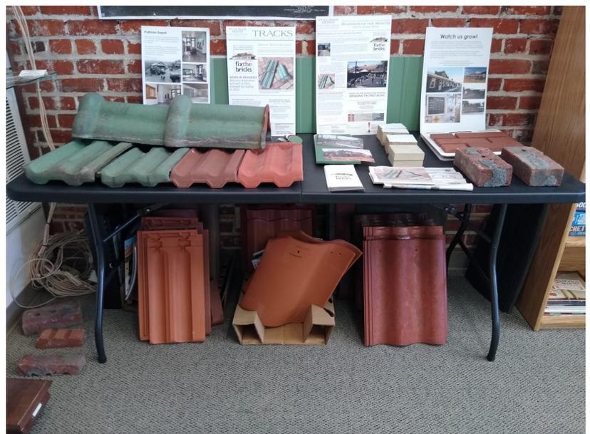
Room, you can hold samples of the original roof and its potential replacements in your own hands. The old terra cotta has an impressive weight and strength to it that are undiminished by its age. It is cool to the touch, and you can still feel the solid earth it is made of. The composite varieties, by contrast, feel like little more than injection plastic, and it is indeed hard to believe it would last as long or perform as well. Several metal roofing options can also be viewed.
